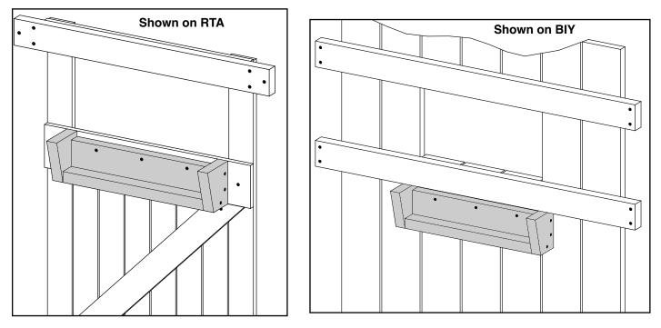
*Note:* You will want to locate flower box where there are thicker boards and the 2½" deck screw does not protrude through the backside.
